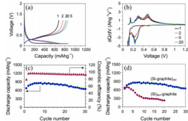
**Figure 4.** Voltage profiles (a), their differential capacity plots (b) and cycling ability of the lithium cells with (c) Si-graphite composite electrode with an artificial SEI, and (d) composite electrode consisting of Si with an artificial SEI and bare graphite in the presence of TMVS, as a function of cycle number.
