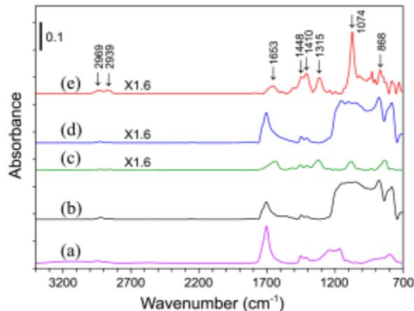
**Figure 3.** IR spectra for (a) polyacrylic acid binder, and the surface of (b) pristine Si electrode and (c) that after five cycles in the presence of TMVS additive, and (d) pristine Si electrode with an artificial SEI of siloxane network and (e) that after five cycles in the presence of TMVS.
